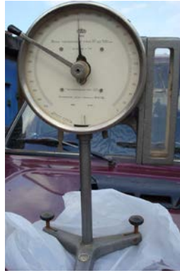
Fig. 2 Torsional Weighing Machine Produced in Poland. Measurement error does not exceed 1 mg.
