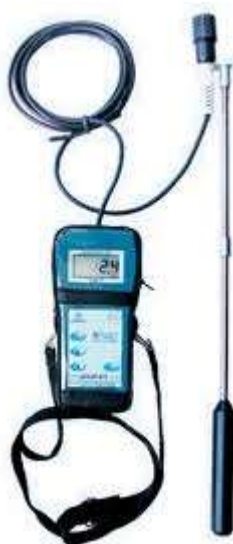
Fig. 2 Gas indicator Dozor S-P
