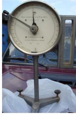
Fig. 2 Torsional Weighing Machine
