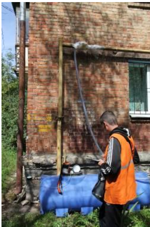
Pic. 4. Monitoring measurement of methane leaks on the ball valve, register number 2525 (Scherbakova str., 62-A).
