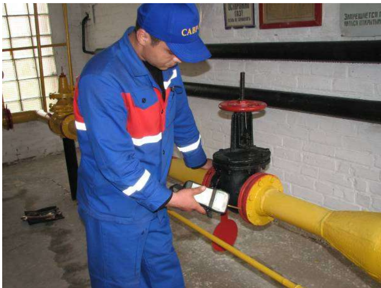
Figure 2. Measurement using gas analyzer DOZOR-S-P.
