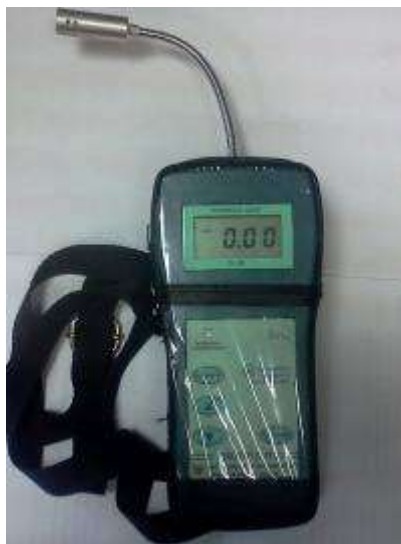
Figure 3. Gas Analyzer DOZOR-S-P
