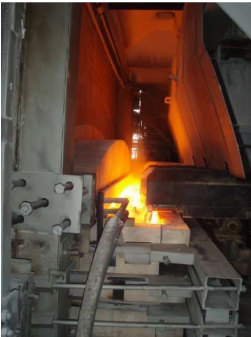
Fig. 6. Batch feeder assembly at the furnace in workshop № 3.
