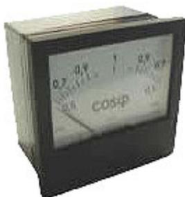
Fig. 4. Typical phase meter
