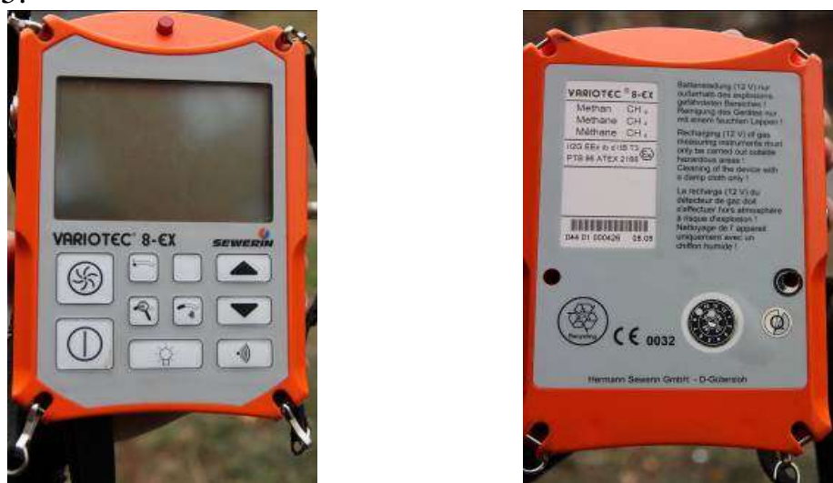
Figure 5. A photo of Variotec® 8-EX gas analyzer.
