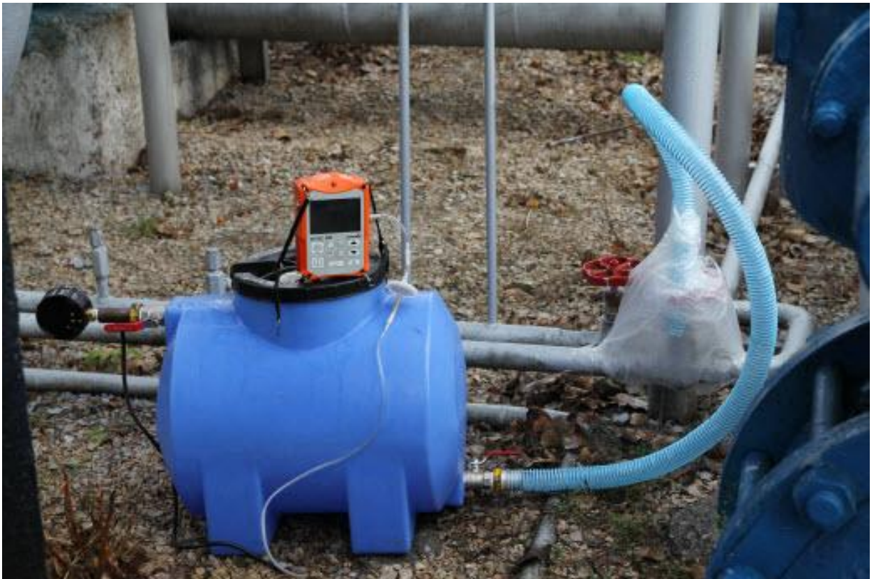
Figure 1. Photo of installation for quantitative measurement of methane leaks
