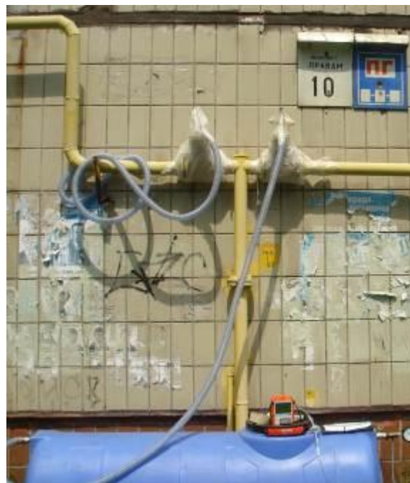
Pic. 4 Monitoring measurement of methane leaks on the wedge latch register number 3032 (Avenue Pravda, 10).
