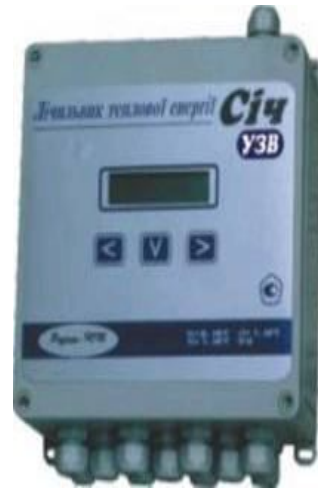
Figure 4. Heat and water meter (СІЧ-УЗв)
