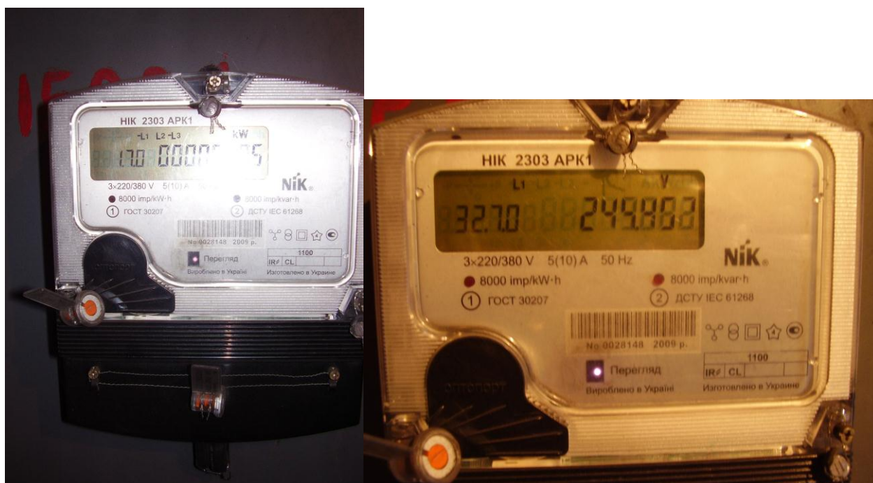
Figure 2 Electricity meter “NIK 2303ARK1”
