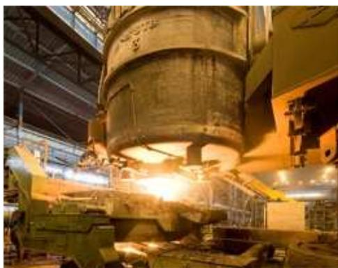
The use of EAFs allows steel to be made from 100% scrap metal feedstock. Therefore, the primary benefit is the substitution of virgin iron which requires much energy to be produced, with scrap that has no emission as it is waste. It is also significant that there is a large reduction in specific energy (energy per unit weight) required to produce steel. In addition, modern EAFs are more flexible, being able to vary production to meet
